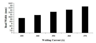
Figure 1: Effect of Welding Current on Weld Bead Width
