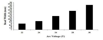
Figure 2: Effect of Arc Voltage on Weld Bead Width
